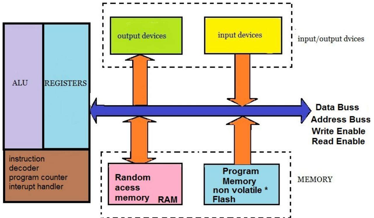
Figure 3: Microprocessor Block Diagram
